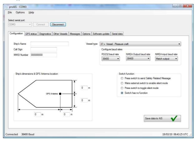
6. The functions of proAIS are arranged in a series of tabs. Each tab contains information relating to a particular aspect of the connected AIS transponder. Depending on the version of proAIS installed not all tabs shown below may be visible.
