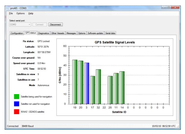
Satellite signal strength bars are shown in green for satellites that are currently being used for navigation. Blue signal strength bars are used to show satellites not currently being used for navigation. It is normal for the graph to display a combination of green and blue bars.
